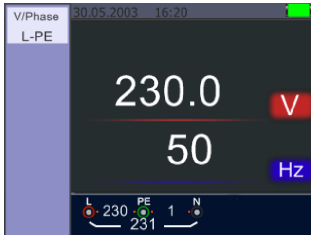
Figure 20 Screen while measuring Voltage and Frequency
