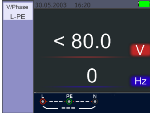
Figure 19. Standby screen for the Voltage and Frequency
