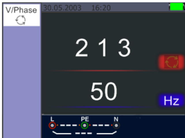
Figure 24 Phase Sequence – When connected in counter-clockwise manner
