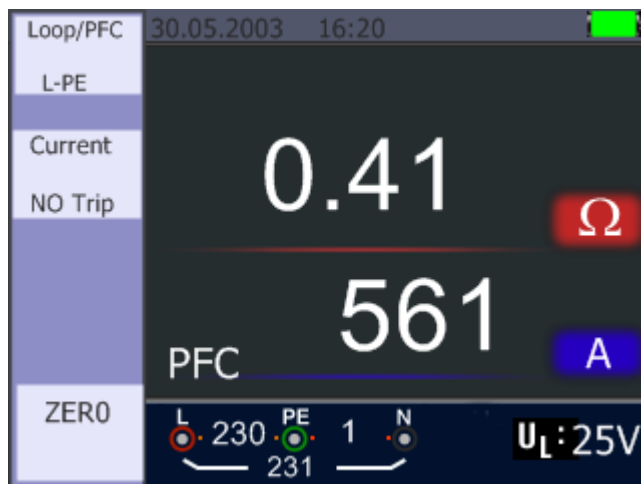
Figure 5 No Trip – Measurement completed
