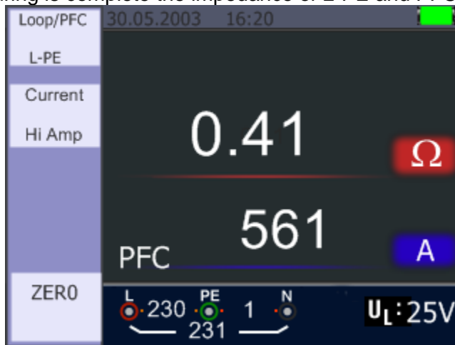
Figure 9 Hi Amp LOOP – Measurement finished
