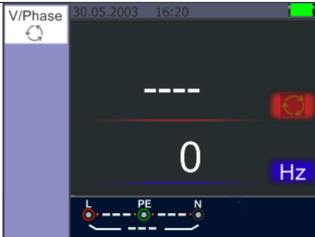
Figure 21 Initial screen of the Phase Sequence Measurement
